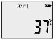
Single press any button or to wake the device, "READY" means logger is OK for a start. The battery indicates the power of the logger.
